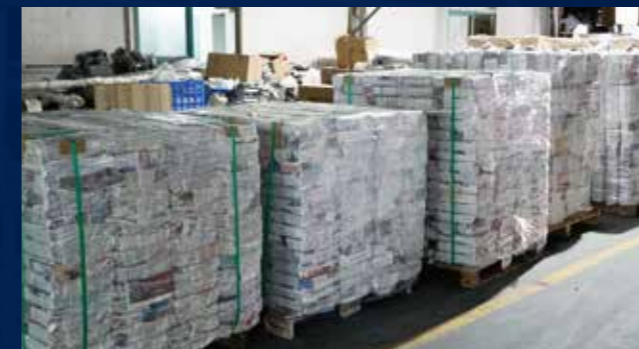
Single wrapped newspaper + electrostatic film + wooden support
