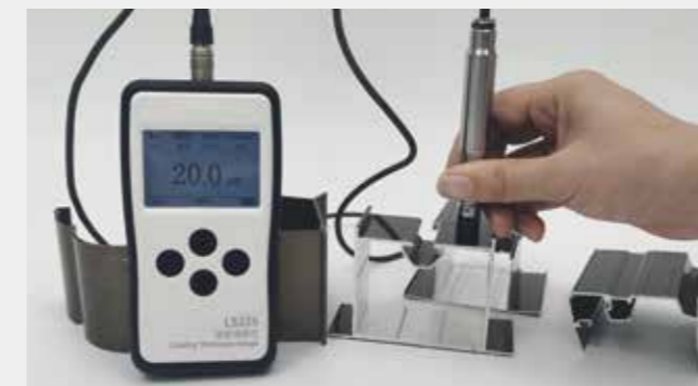
Testing Powder Coating Surface
