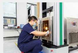
隔热条高低温性能测试 Insulation strip high and low temperature performance test
