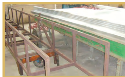
装料框未加工 (未保护) Iron rack without felt protection (unprotected)
