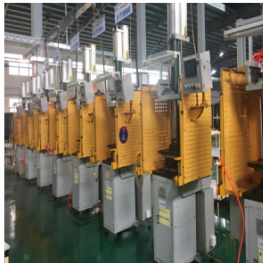
15吨注射密封条接角机 15 Tons Sealing Strip Injection Angle Machine
