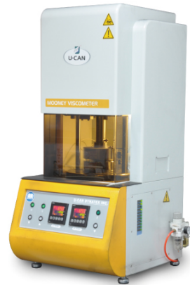
门尼粘度仪：用于测定生胶或混炼胶的门尼粘度值、焦烧时间。 Mooney Viscometer: detect Mooney viscosity and scorch time of raw rubber or rubber compound
