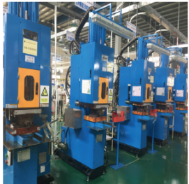
30吨注射密封条接角机 30 Tons Sealing Strip Injection Angle Machine
