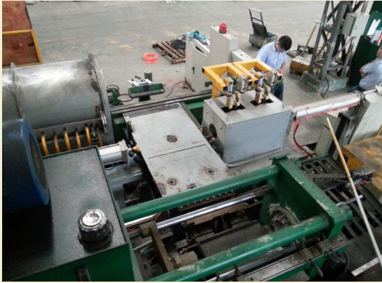
隧道式短棒燃气炉配变频梯度加热炉 Tunnel type short bar gas furnace equipped with variable frequency gradient heating furnace
