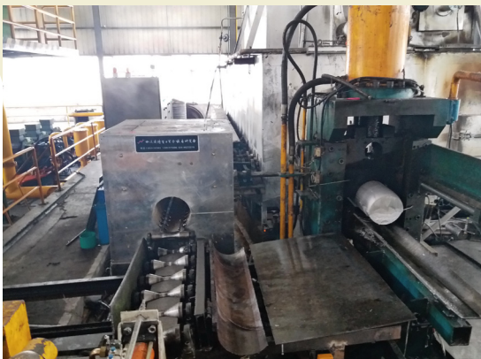
长棒热剪炉配变频梯度加热炉 Long bar hot shear furnace equipped with variable frequency gradient heating furnace
