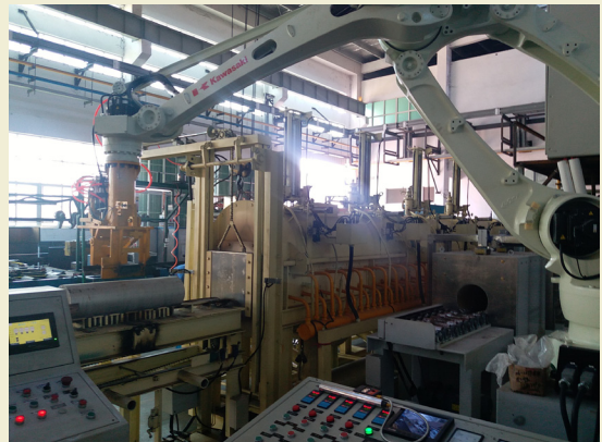
机器人燃气加热炉配变频梯度加热炉 Round type gas heating furnace equipped with variable frequency gradient heating furnace
