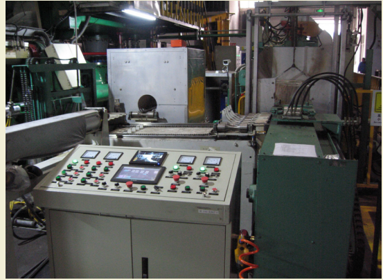
隧道式短棒燃气炉配变频梯度加热炉 Tunnel type short bar gas furnace equipped with variable frequency gradient heating furnace
