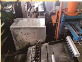
可配套热后梯度加热 The clipping machine of hot aluminum bar
