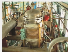
变频不锈钢加热炉 Induction heating furnace for stainless steel heating
