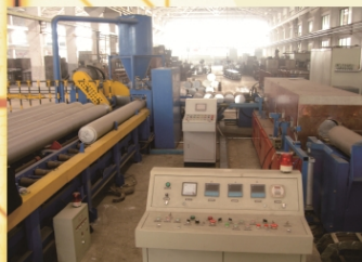
228mm铝棒变频梯度加热炉配有线锯 228mm Aluminum Bar Frequency Conversion Induction Gradient Heating Furnace with On-line Saw
