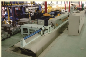
254mm铝棒变频梯度加热炉 254mm Aluminum Bar Frequency Conversion Induction Gradient Heating Furnace
