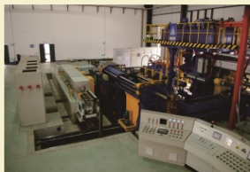
254mm铝棒变频梯度加热炉用于新马铝业公司 254mm Aluminum Bar Frequency Conversion Induction Gradient Heating Furnace
