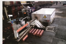
变频铜加热炉 Induction heating furnace for copper bar
