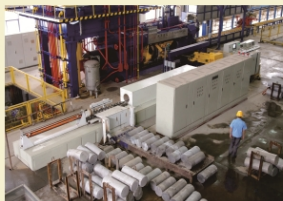
350mm铝棒变频梯度加热炉 350mm Aluminum Bar Frequency Conversion Induction Gradient Heating Furnace
