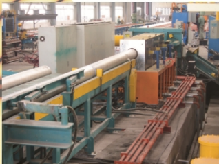
可配套长棒料加热剪切机构 The deliver machine of long aluminum bar
