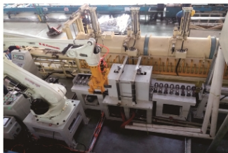
燃气预热后单棒多温区梯度加热炉 Gas preheating Induction Multi-temperature Zone Gradient Heating machine
