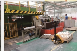
变频银加热炉 Induction heating furnace for silver bar
