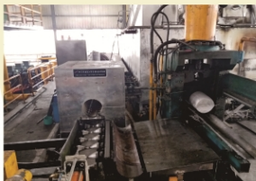
254mm铝棒热剪后变频梯度加热炉用于盛达光亮铝业公司 Frequency Conversion Gradient Heating Furnace for 254 mm Aluminum Bar after Hot Shearing
