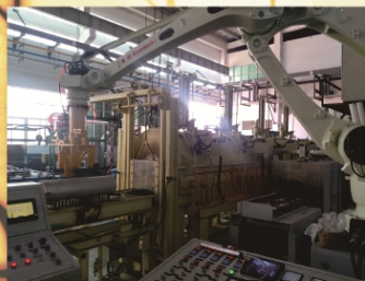
228mm铝棒变频梯度加热炉用于广东新会铝业铝材有限公司 Induction gradient Heating Furnace after Gas Preheating by Robot Transmission
