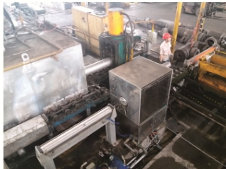
可配套用于燃气加热后变频梯度加热 The clipping machine of hot aluminum bar
