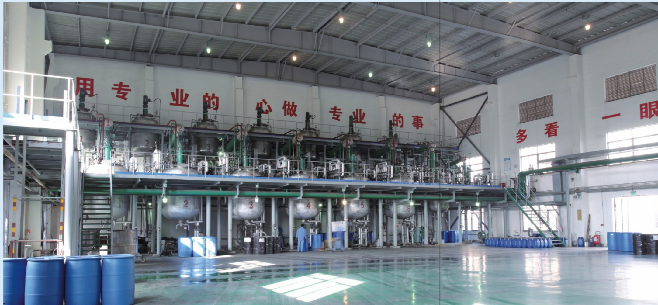
PLC电脑全自动电泳涂料生产线 Computer automated PLC production line
