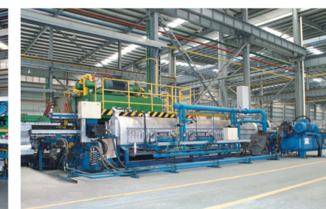
长棒加热炉及热剪机 Long rod heating furnace and heat shearing machine
